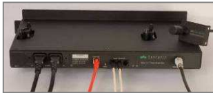
Connect dual power, network, remote sensors
